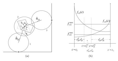
Figure 1: The collision geometry (a), and dependency of collision modes on c (b)
