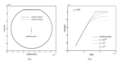
Figure 4: Phase plane of sphere's motion (a) and vel. at stick-slip transition (b)
