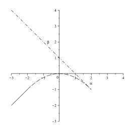
FIGURE 1. In this Figure, we have plotted the area in the  $(\alpha, \beta)$ -plane where  $|\lambda_1| < 1$ . The domain is bounded by the line  $\alpha + \beta = 1$  which is plotted using a dashed and dotted line, the parabola:  $\alpha^2 + 4\beta = 0$  which is plotted using a dashed line, and  $\beta - \alpha = 1$  which is plotted using a solid line.
